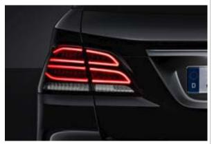
H7 Halogen headlamps paired with bright white LED Daytime Running Lamps help increase the visibility of your vehicle to oncoming traffic. The taillamps feature a fiber-optic dual "torch" design and LED turn signals and brake lamps.
